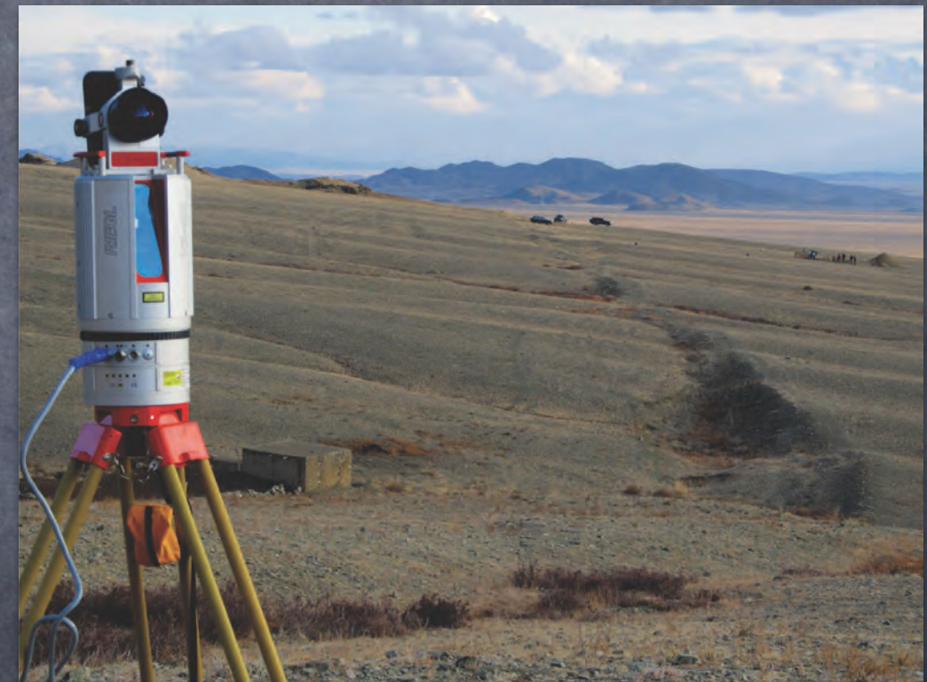
Lidar sol (Laser Detection And Ranging)
